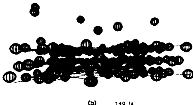
Fig. 1. Positions of the atoms. (a) Before the primary ion (the lone sphere above the solid) has struck. (b) Consequences of a single ion impact. The two atoms being ejected to the left form a dimer. For clarity, only a selected group of atoms is shown, and their size is arbitrarily drawn. The elapsed time during the collision is shown in femtoseconds ( 1 \text{ fs} = 10^{-15} second).
