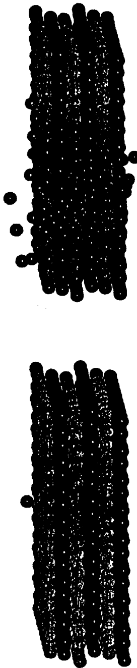
Figure 5. Positions of the atoms in a Rh(111) surface before and after 3-keV Ar ion bombardment. In the final positions the Ar ion appears near the center of the crystal. This trajectory was chosen at random. In some cases there is considerably more atomic motion and in some cases less.
