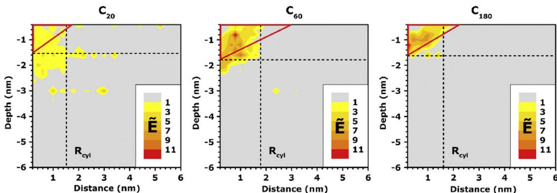
Fig. 2. Energy deposition profiles of 15 keV  $C_{20}$ ,  $C_{60}$  and  $C_{180}$  projectiles bombarding a clean surface of Ag{111} at normal incidence. The figure gives the value of dimensionless parameter  $\tilde{E}$  (see text) at the time when 90% of the energy has been deposited. The dashed lines represent the estimate of  $R_{cyl}$ . The triangle depicts a crystal volume that will contribute to ejection of silver atoms estimated from the MEDF model [9].
