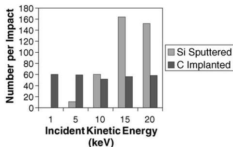
Fig. 1. Number of C atoms implanted and number of Si atoms sputtered from  $C_{60}$  keV bombardment of Si at normal incidence.
