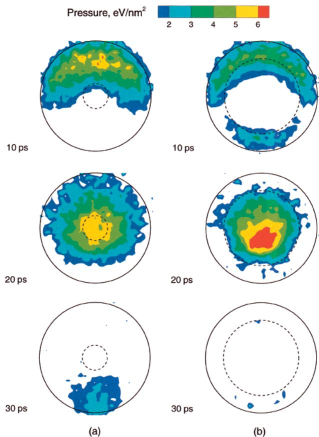
Figure 8. Spatial distribution of the 2D pressure within the particles that contain small (a) and large (b) transparent inclusions. Simulations are performed at a laser fluence of 300 eV/nm. The solid and dashed circles show the original boundaries of the particles and inclusions, respectively.
