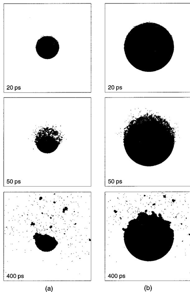
Figure 2. Snapshots from the simulations of laser irradiation of small, 50 nm in diameter, particle (a) and large, 110 nm in diameter, particle (b). The laser penetration depth is 25 nm, the pulse duration is 15 ps, and the laser fluence is 25 eV/nm. Snapshots are shown for times 20, 50, and 400 ps after the start of the laser pulse.
