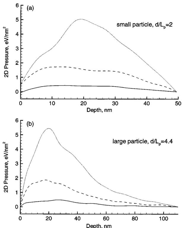
Figure 5. 2D pressure versus depth into the particle for the small particle (a) and the large particle (b). The pressure is averaged for the middle 10% of the particles at 10 ps after the start of the laser pulse. Zero value of the depth corresponds to the front edge of the illuminated side of the particle. The solid, dashed, and dotted lines are for the simulations with laser fluences of 25, 100, and 300 eV/nm, respectively.
