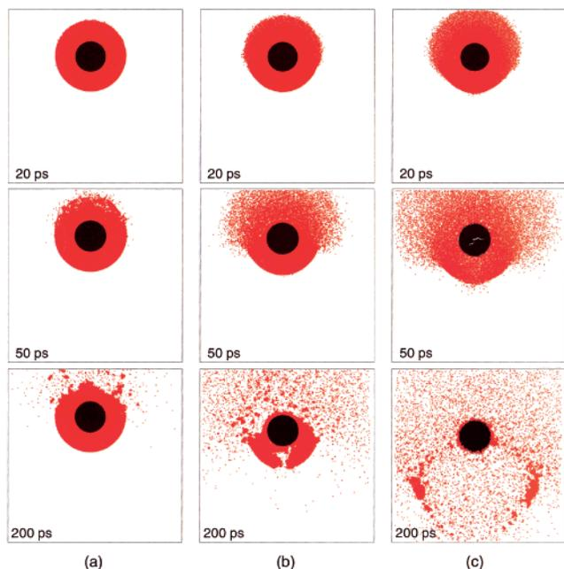
Figure 6. Snapshots from the simulations of laser irradiation of particle with a transparent inclusion of medium (45% of the particle diameter) inclusion. Snapshots are shown for times 20, 50, and 200 ps after the start of the laser pulse. Simulations are performed with laser fluences of (a) 25, (b) 100, and (c) 300 eV/nm. Absorbing molecules are red; molecules that belong to the transparent inclusion are black.
