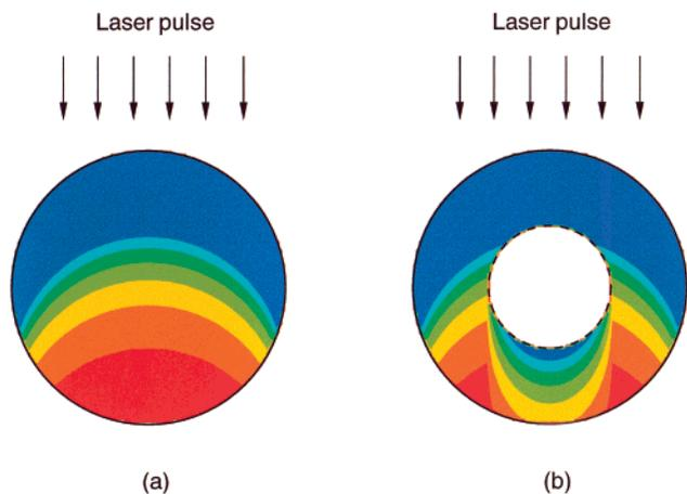
Figure 1. Schematic drawing of the energy density distribution in a homogeneous absorbing particle (a) and a particle with a transparent inclusion (b) irradiated by a laser pulse. The energy density is the highest in the blue areas and the lowest in the red areas. The transparent inclusion is marked by the dashed line. For the circular geometry, the distance  $z = 0$  for Beer's law is the semicircular front edge of the particle. The size of the particle is 110 nm with a 50-nm core for frame b.
