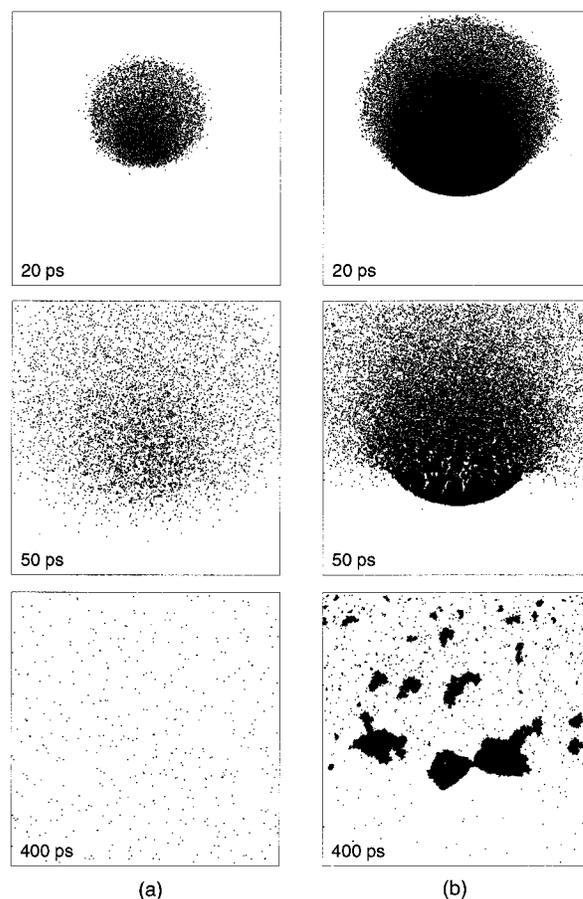
Figure 4. Same as in Figure 2, but for a laser fluence of 300 eV/nm. The area shown in the snapshots taken at 400 ps is shifted down by 200 nm to show the clusters in (b) that are moving with velocity of  $\sim 500$  m/s in the direction of the laser pulse.
