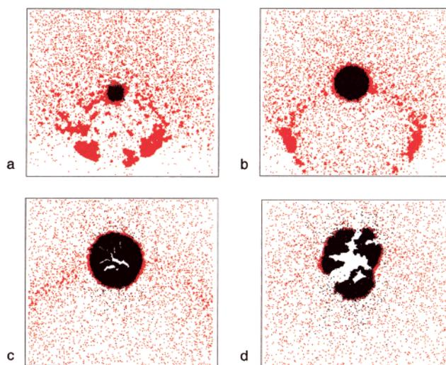
Figure 7. Snapshots from simulations performed for particles with transparent inclusion of three different sizes, (a) small (23% of the particle diameter), (b) medium (45%), and (c, d) large (68%). A laser fluence of 300 eV/nm is used in the simulations illustrated by snapshots in (a–c) and 500 eV/nm in (d). Snapshots are shown for 200 ps after the start of the laser pulse. Absorbing molecules are red; molecules that belong to the transparent inclusion are black.
