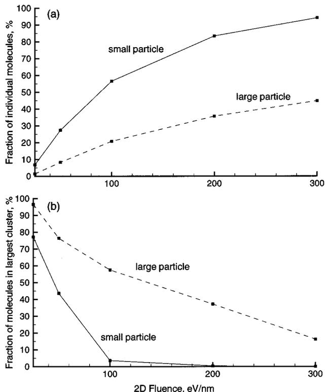
Figure 9. Fraction of individual molecules (a) and molecules in the largest cluster (b) calculated at the end of the simulations, 400 ps, for different laser fluences.
