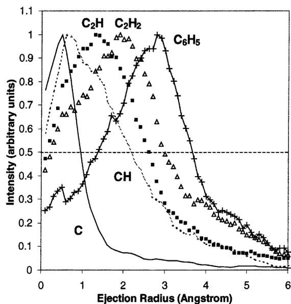
Fig. 3. Calculated distributions of distances between the impact point and the center-of-mass of the nascent fragments obtained from MD simulations (500 eV Ar bombardment of polystyrene tetramers adsorbed on silver).
