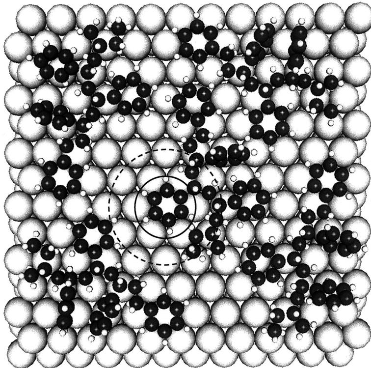
Fig. 1. Top view of the simulation cell used for the bombardment of polystyrene molecules by 500 eV Ar atoms. The full circle corresponds to the calculated ejection area of the phenyl radical and the dashed circle represents the experimental disappearance cross-section of the same fragment.
