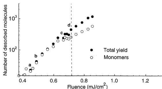
Fig. 1. Total and monomer yields vs. fluence. The dashed line indicates the threshold fluence for ablation.
